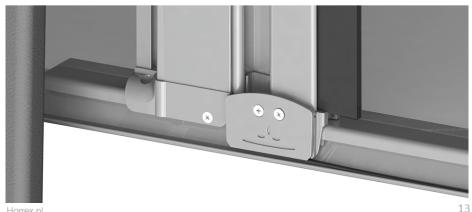
18 insert the cord tensioner as shown. Put the cords under tension by unscrewing the set screw, pulling on the cords and fastening the set screw.
