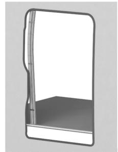
When the cassette is perpendicular to the bottom guider fasten the cassette to the bottom guider.
