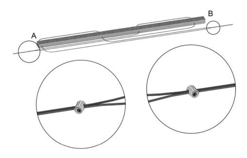
6 Place tape on the back of the mesh pack to insure the cord stays in position.
