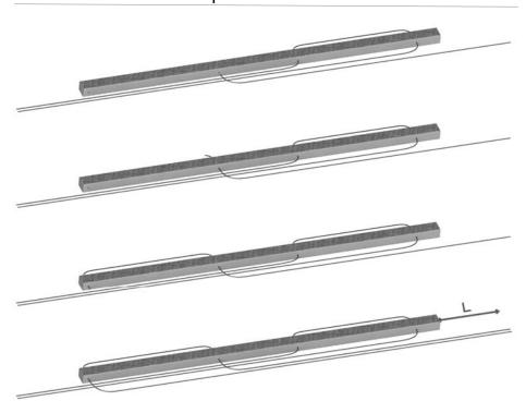
4 Side A is where the cord goes through the mesh pack the closest to the edge. Side B is the other side.
