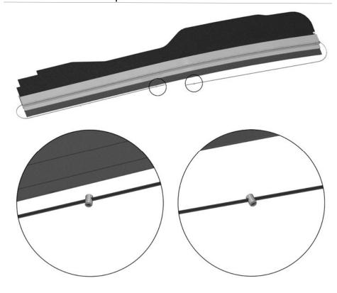
Place the cord in the guider piece and slide the cassette and pullbar in the top guider.
