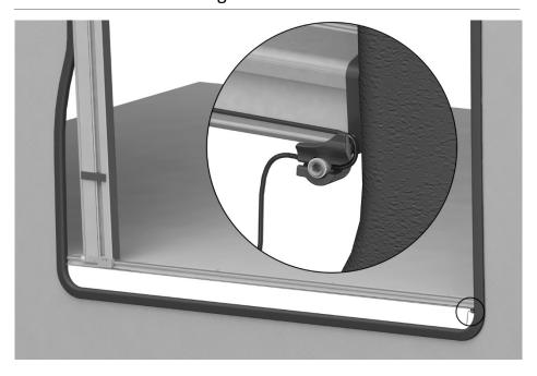
Position the top cord tensioner into the top profile endcap.
